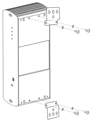
Once the bracket mounting is secured onto the extender, it is ready for mounting onto a surface. Please note you will need to provide your own screws to secure the extender using the available slots on each bracket.
