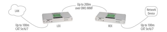
Connect any network device or access port into the RJ45 socket label "LAN" using up to 100 meters of standard CAT 5e, 6 or 7 cabling.
