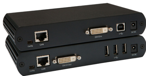
Rear views of local extender (top) and remote extender (bottom)
