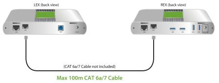
2 Connect the LEX to the computer's USB 3 port using the included USB cable.
