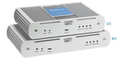
Icron's next generation USB 3-2-1 extender, the Raven 3204C extends USB 3 (5Gbps), USB 2.0 and USB 1.1 devices up to 100m (330 ft) from a host computer across a point-to-point CAT 6a/7 connection. The Raven 3204C delivers the same exceptional performance as the Raven 3104, in a smaller, lighter design, with USB-C ports available for the host and extended devices.
