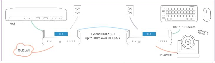
\* If the host computer can deliver 15W to the LEX, the LEX power supply is not required.
