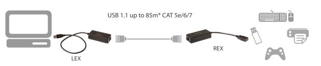
\* Up to 40m for all USB devices; 85m is achievable for most low powered HID USB devices.
