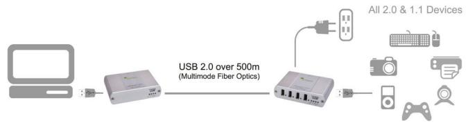
USB extension up to 500m over fiber optic cable
