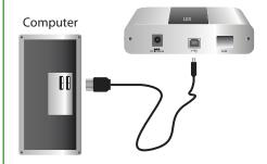
Note: Power adapter is not required at the LEX for normal operation.
