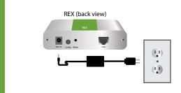
4 Attach the USB device(s) to the REX.
