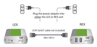
Note: Flexible power is different from Power over Ethernet (PoE). Ensure the CAT 5e/6/7 cable is only connected between the LEX and REX units.
