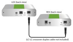
Max 500m multimode fiber for RG2324 Max 10km singlemode fiber for RG2344 2 Connect the LEX to the computer using the included USB cable.
