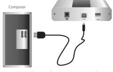
Note: Power adapter is not required at local extender for normal operation.
