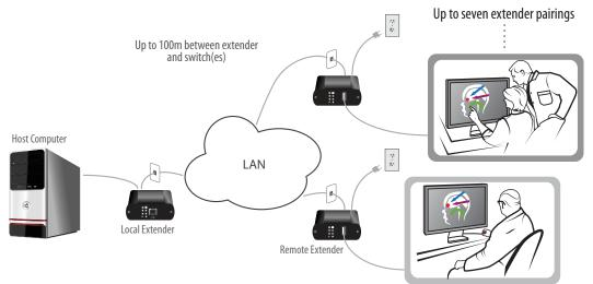
\* Maximum throughput will vary based on network traffic, distances and number of switches between extenders.
