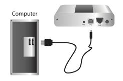
3 Connect the Remote Extender to the AC adapter and a power source.
