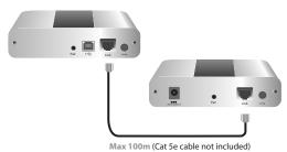
Connect the Local Extender to the computer using the included USB cable.
