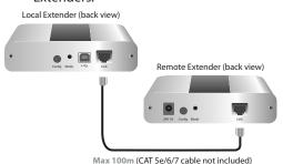
Connect the Local Extender to the computer using the included USB cable.
