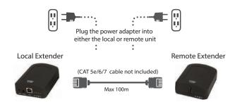
Connect the Local Extender into your computer using the included USB 2.0 cable.
