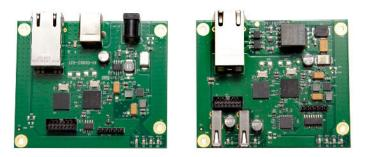
LEX/REX Turnkey 2212 extends USB 2.0 beyond the desktop up to 100m over standard Cat 5 cable using ExtremeUSB<sup>®</sup> technology.
