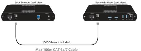
2 Connect the Local Extender to the computer's USB 3 port using the included USB cable.
