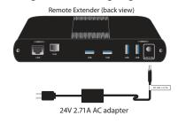
5 Attach USB device(s) to the Remote
