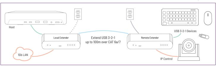
\* If the host computer can deliver 15W to the Local Extender, the Local Extender power supply is not required.
