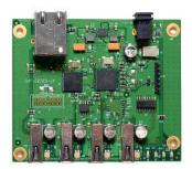
LEX/REX Turnkey 2204 extends USB 2.0 beyond the desktop up to 100m over standard Cat 5 cable using ExtremeUSB® technology.
