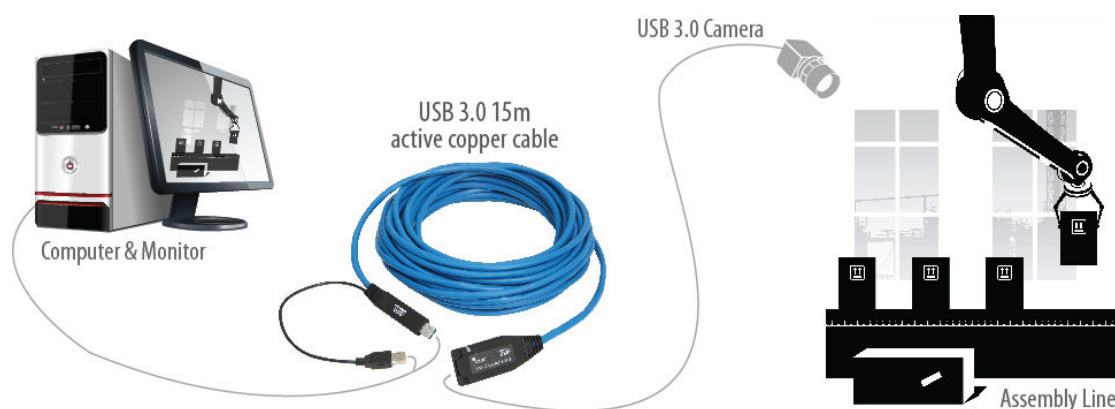
Figure 2 - Extending a Machine Vision Camera 15m with Icron's USB 3.0 Spectra™ 3001-15 Active Cable
