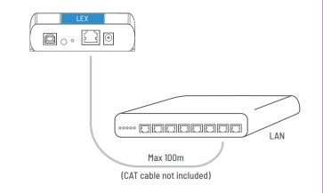
Place the REX where desired. Connect a CAT 5e/6/7 patch cable to the RJ45 Link port on the REX and to an IEEE 802.3at - PoE+ (25.5W) capable LAN port.
