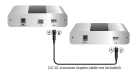
Max 500m multimode fiber for RG2224 Max 10km singlemode fiber for RG2244
