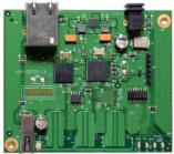
LEX/REX Turnkey 2201 extends USB 2.0 beyond the desktop up to 100m over standard Cat 5 cable using ExtremeUSB® technology.
