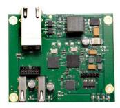
LEX/REX Turnkey 2212 extends USB 2.0 beyond the desktop up to 100m over standard Cat 5 cable using ExtremeUSB® technology.
